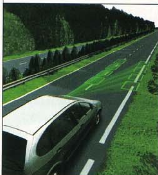
Smart safety system warns drowsy drivers to stay between the lines.
